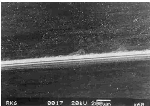
Fig. 7. Edge machined by grinding a sample containing 22.5 wt.% binder.
